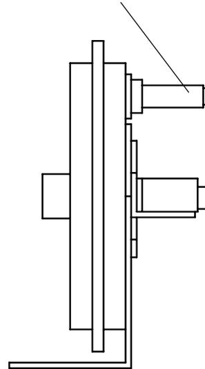
Figure 6. Draft Proving Switch
