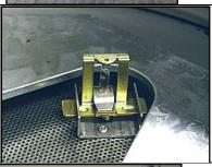
9. Replace the gasket and burner access door assembly. (Note door gasket color may vary.)
