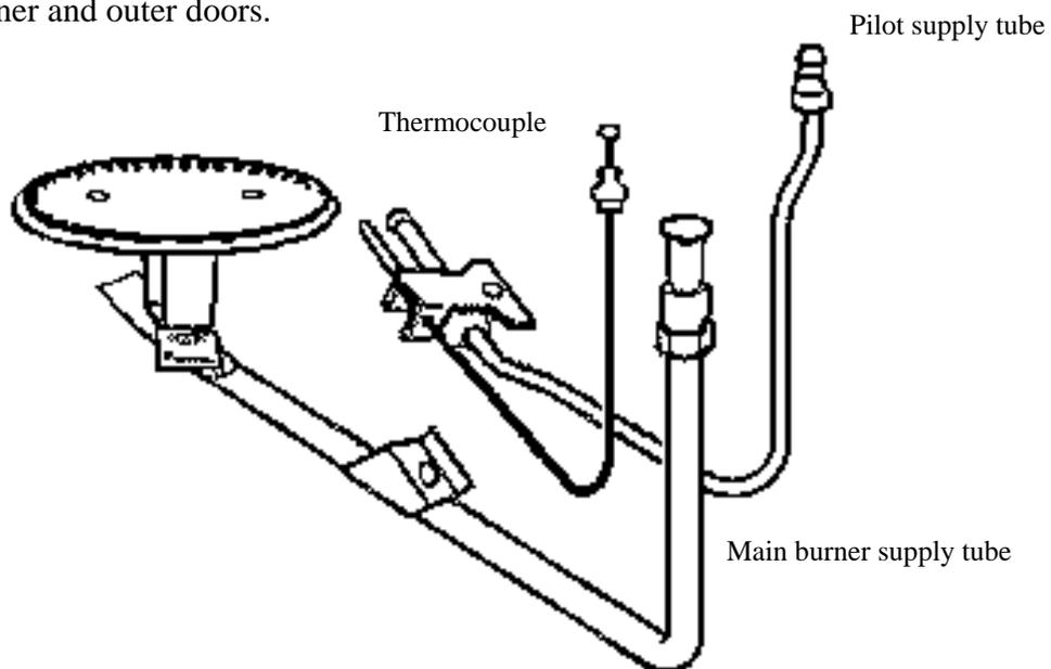
Maintenance Tip: While the burner assembly is out of the combustion chamber, take the time to clean and vacuum the combustion chamber. Brush and clean the burner plate and orifice. Look for signs of rust and sooting.
