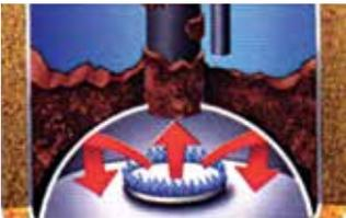
Sediment build-up in a water heater creates layers of non-conducting material between the water and the energy that heats the water. This causes a reduction of heat transfer which increases tank bottom temperatures and decreases water temperatures. When this occurs, the results are decreased water heater efficiency and decreased tank life.
