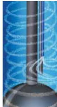
The spiraling effect also creates better mixing throughout the water heater tank which reduces the effects of stacking. Stacking occurs when frequent small draws of water create different temperatures throughout the tank resulting in increased peak temperatures at the top of the tank. The EverKleen™ system greatly reduces peak temperatures, thus increases first hour deliverability.
